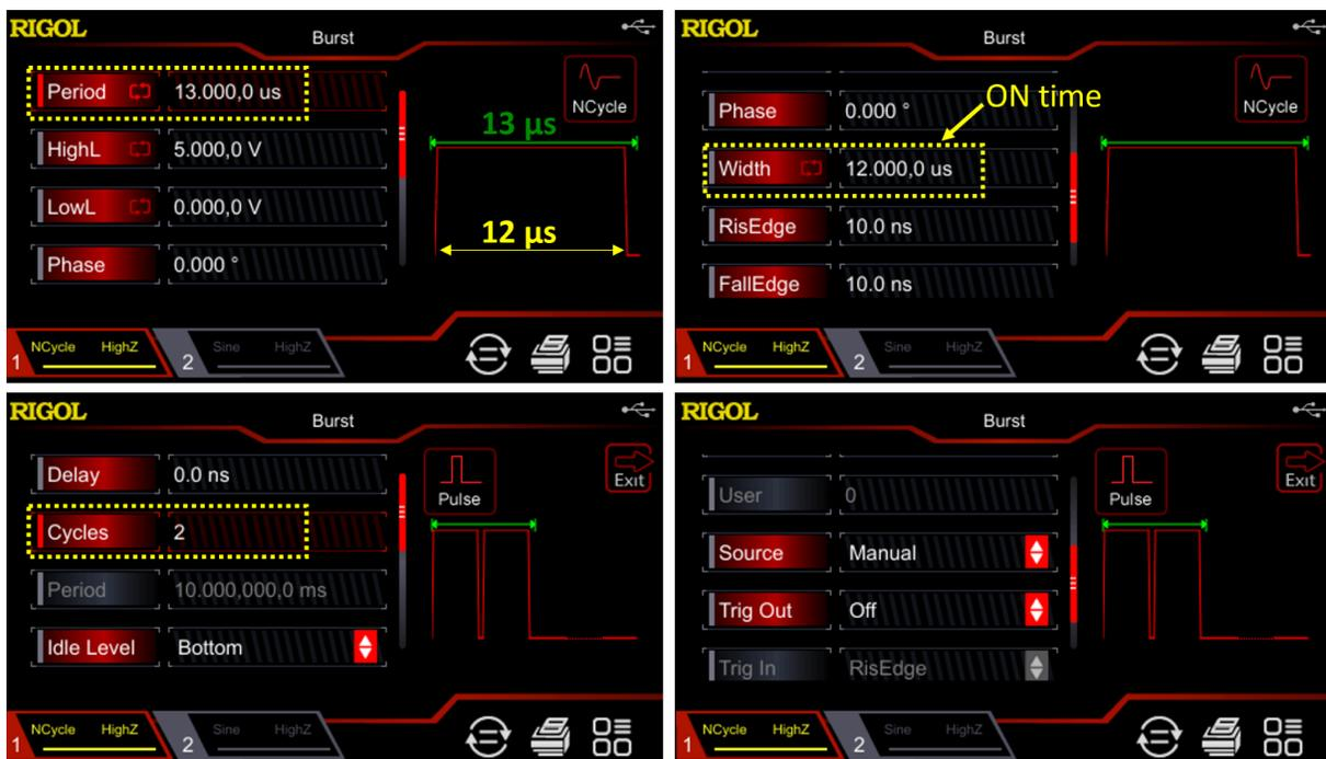
**Figure 4:** Configuration for the PWM pulse signal using the RIGOL waveform generator.
