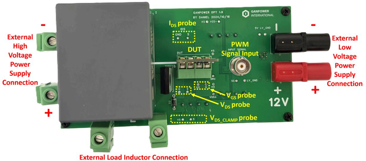
**Figure 2:** GaNPower Evaluation Board Top View.
