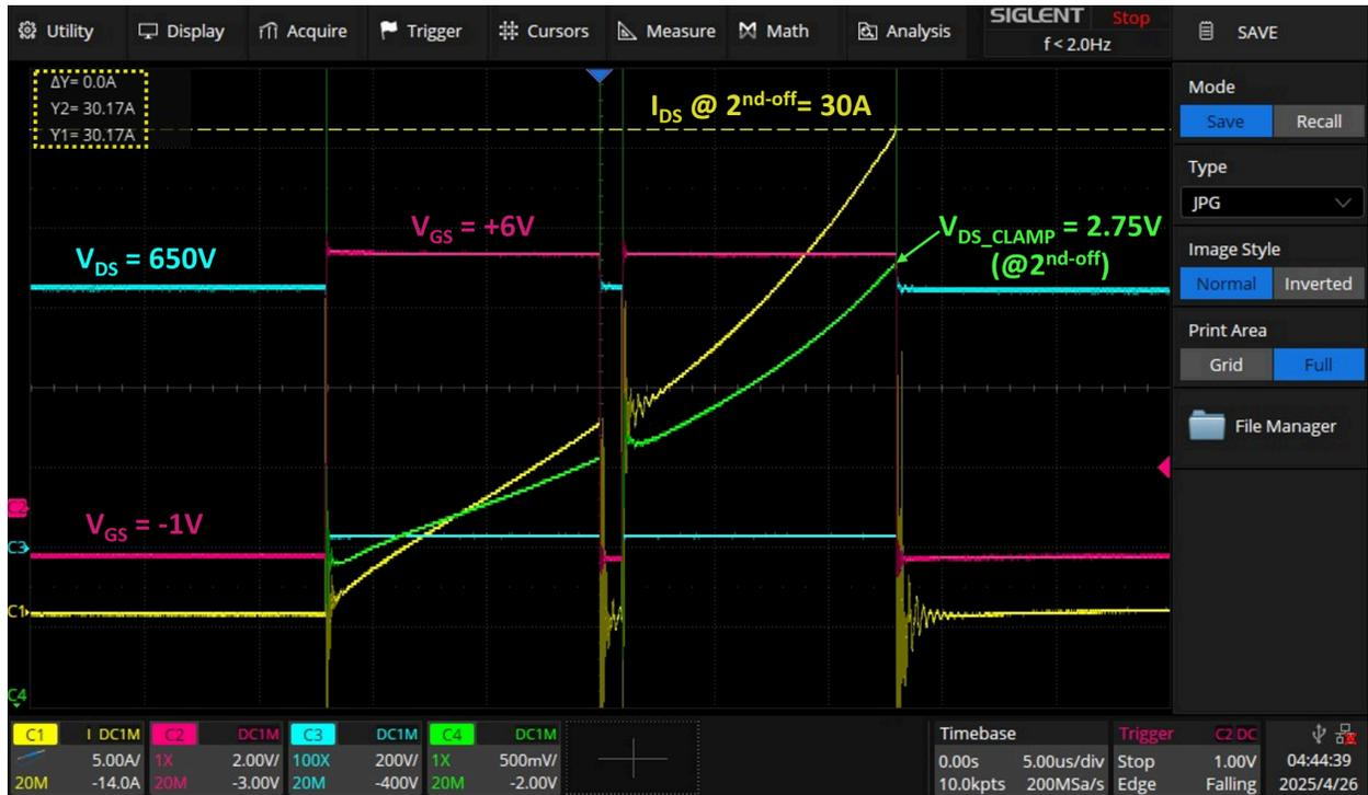
**Figure 6:** DPT of GPI65030DF88 at  $V_{BUS} = 650V$ , with L-load = 360  $\mu H$ .
