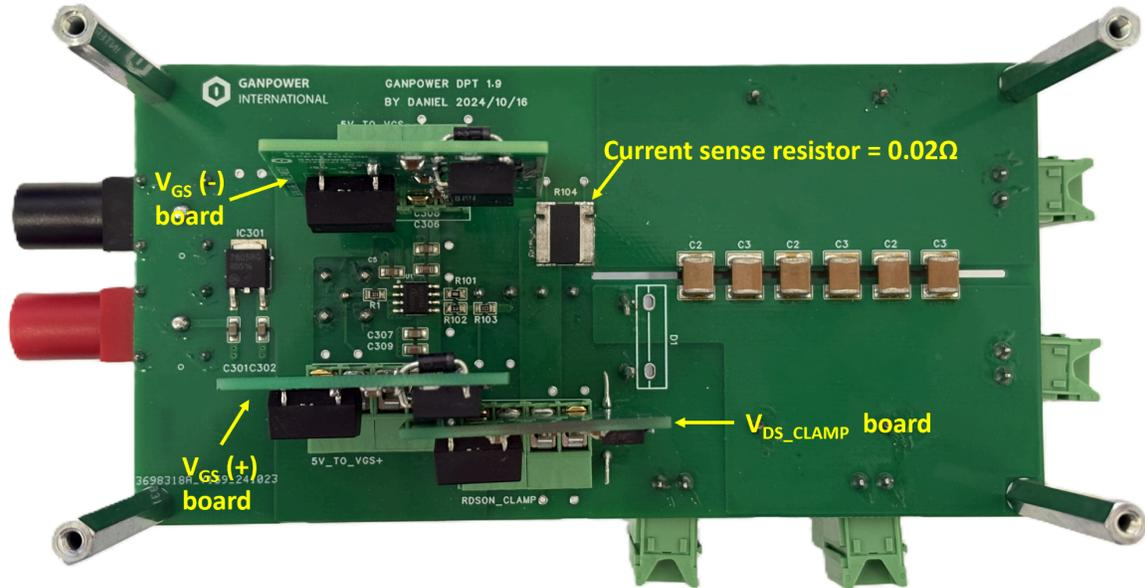
**Figure 1:** GaNPower Evaluation Board Bottom View.
