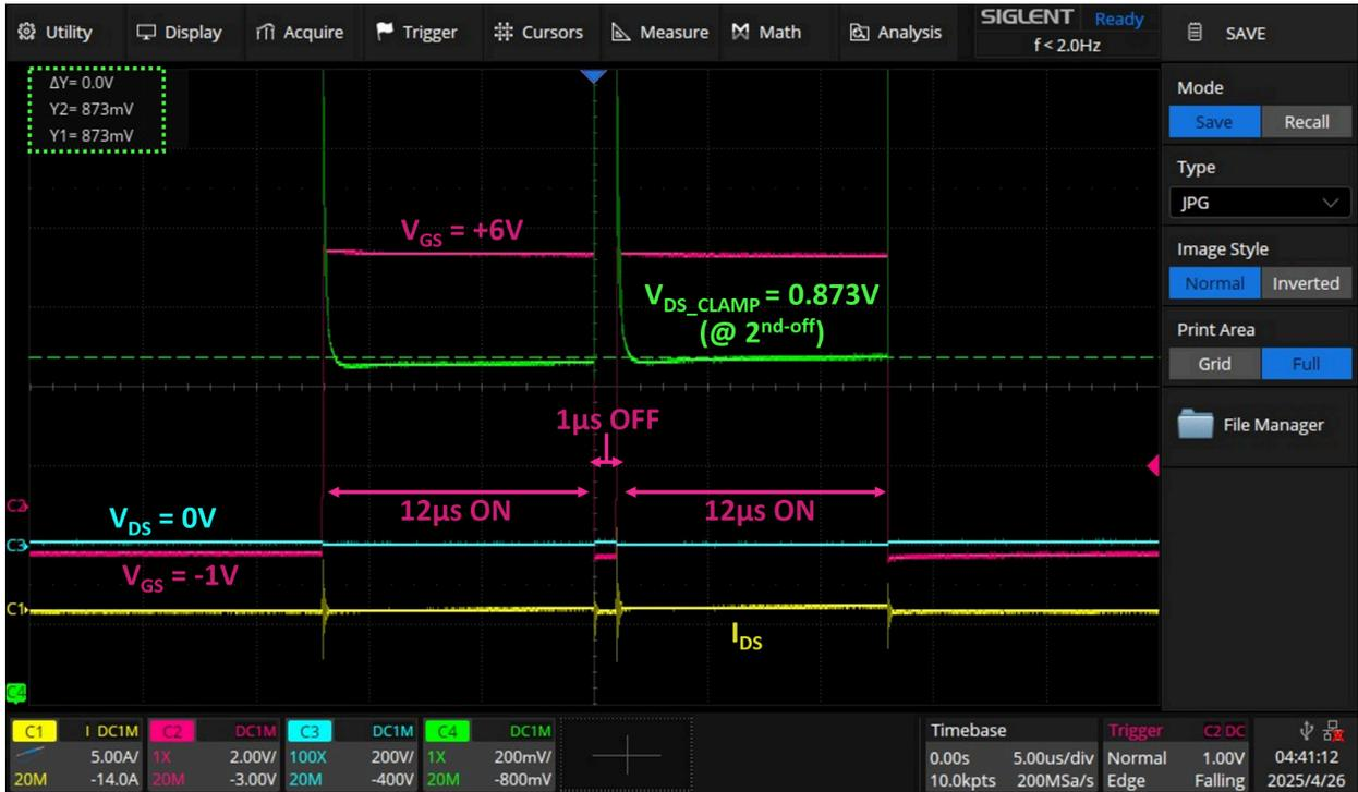
**Figure 5:** DPT of GPI65030DF88 at  $V_{BUS} = 0V$ , showing  $V_{DS\_CLAMP}$  baseline.
