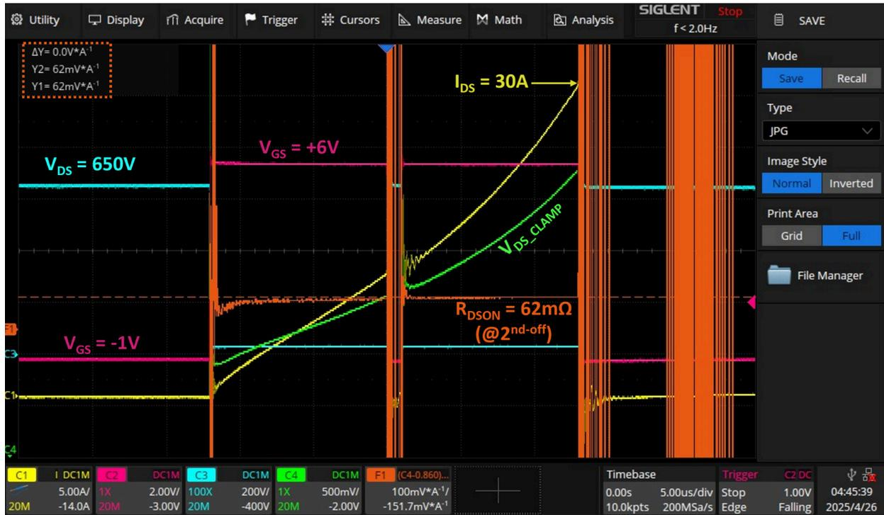
**Figure 7:** DPT of GPI65030DF88 at  $V_{BUS} = 650V$ , illustrating the calculation of dynamic  $R_{DS(on)}$ .
