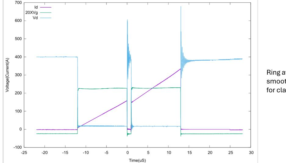
Double pulse testing for bare die packaged within TO247-4. Rgon=2 Rgoff=0. Vg from -1 to 12. Eoff and Eon at 168A are 600uJ and 2350 uJ, respectively. Eoff at 335A is 700 uJ.
