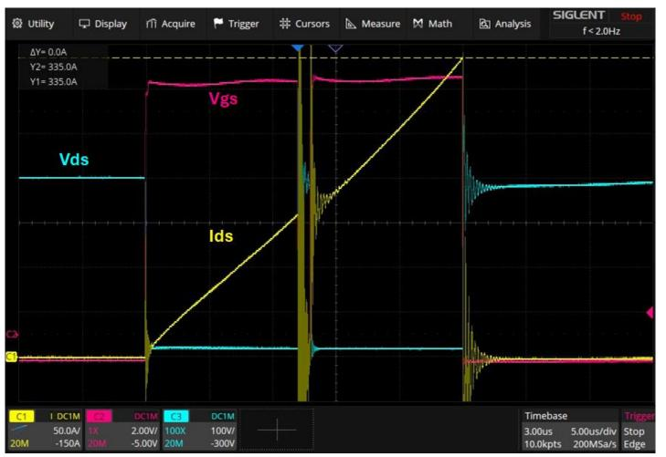
Double pulse testing for bare die packaged within TO247-4. Rgon=2 Rgoff=0. Vg from -1 to 12.
