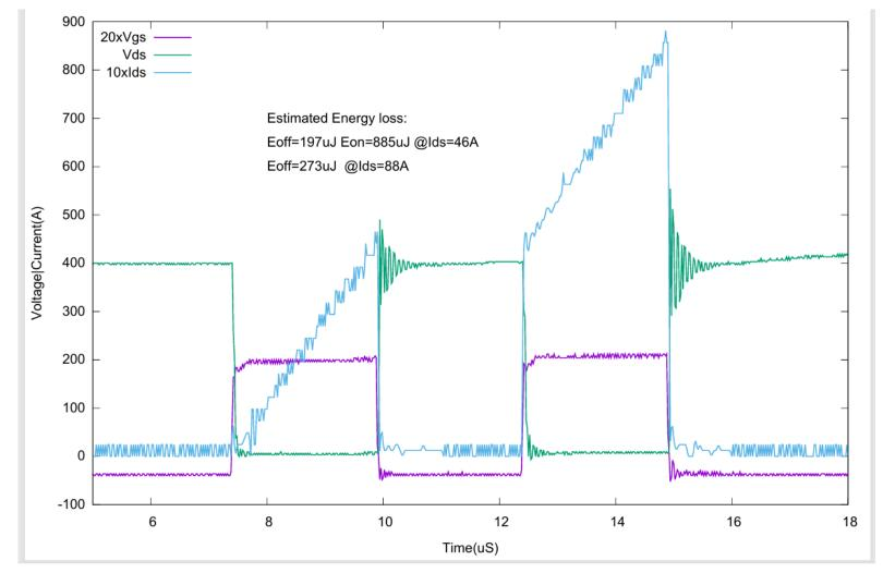
Double pulse testing for bare die packaged within TO247-4. Rgon=10 Rgoff=0. Vg from -2 to 10. Peak to peak averaging method were used for Ids(t) to remove some strong ringing near switching edge in order to estimate Eon/Eoff.
