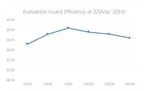
Figure 2. Efficiency at 220V input.
