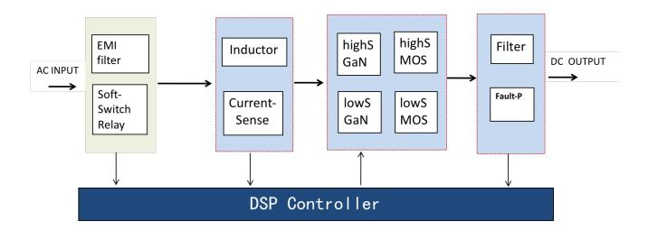
Figure 1 block diagram of the PFC system.
