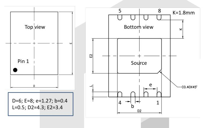
8LEAD DFN(6x8x0.75MM,pitch 1.27 mm) (3.40 x 4.30 mm Exposed area) Bottom thermal pad and Pin 1,2,3=source ; pin 4=gate; pin 5,6,7,8=drain IMPORTANT: Please connect the bottom thermal pad to the source electrode on PCB
